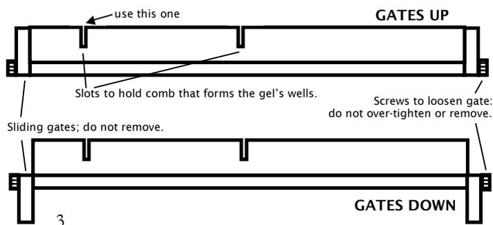
Figure 4. Gel casting tray, side view. Top: gates up. Bottom: gates down.
