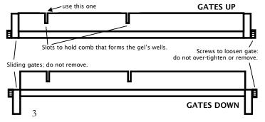
Figure 4. Gel casting tray, side view. Top: gates up. Bottom: gates down.
