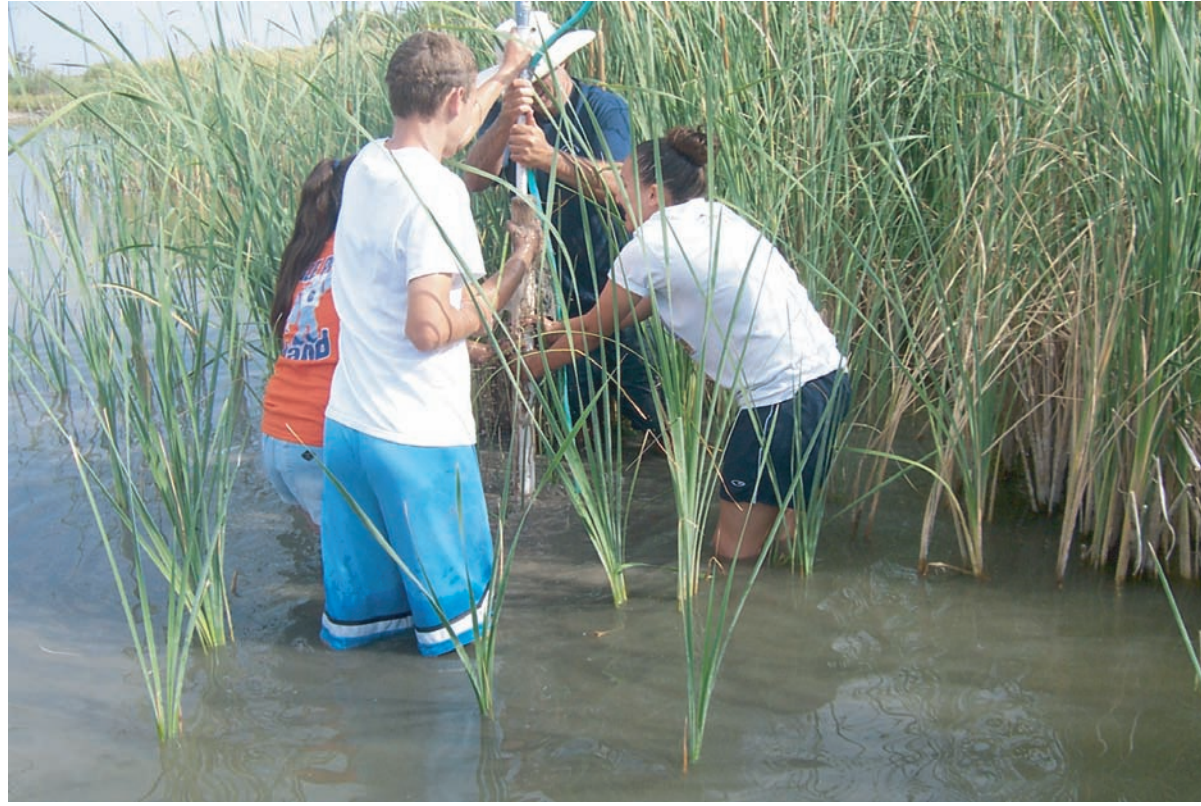
High School Students boring for a piezometer using a hydraulic drill
