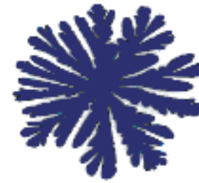
Hele-Shaw cell viscous fingering
