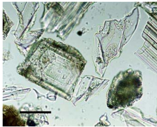
Feldspar mineral surrounded by volcanic glass. Bar scale= 0.05 mm
