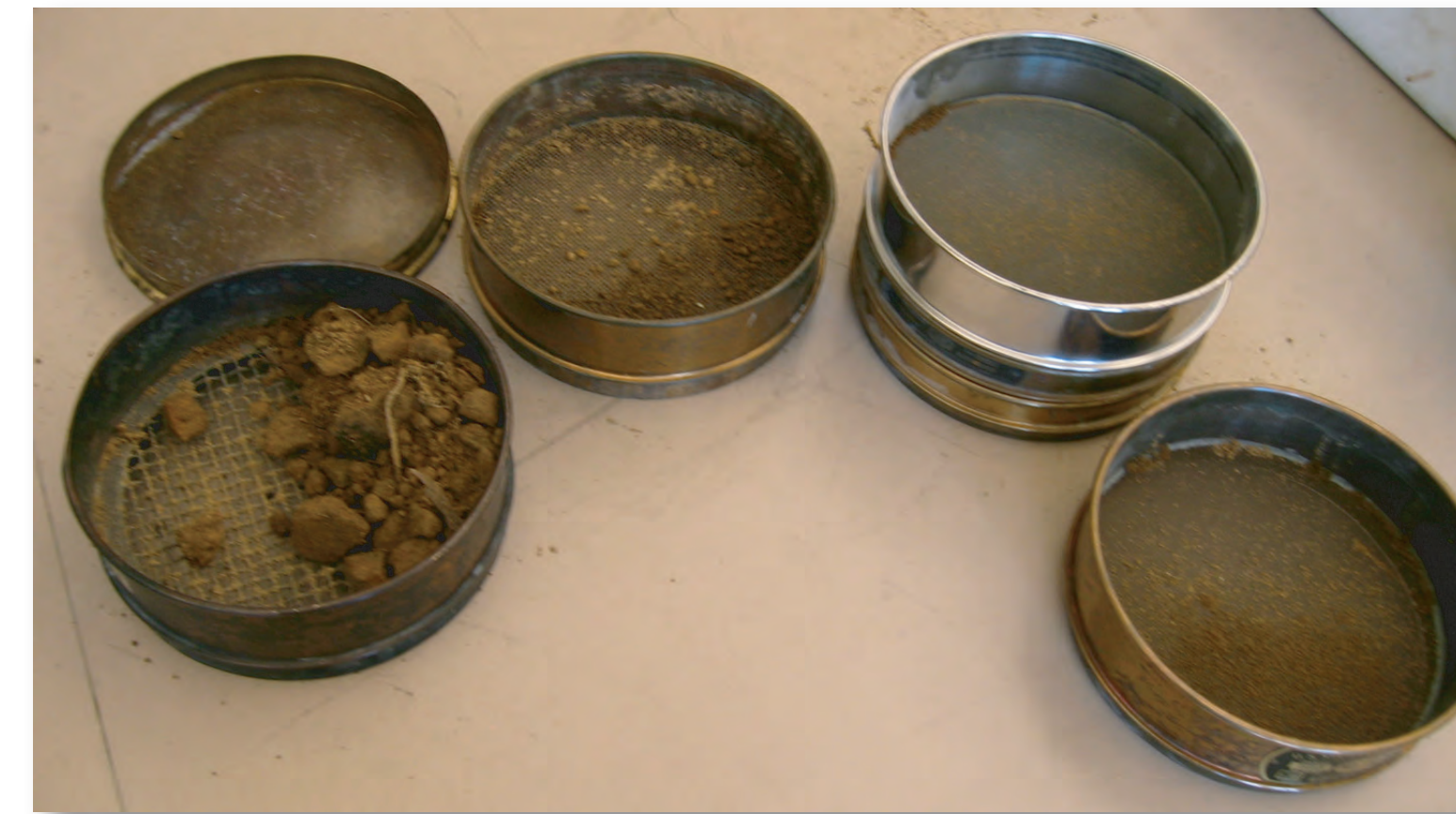
The results of sieving the dried landslide sample
