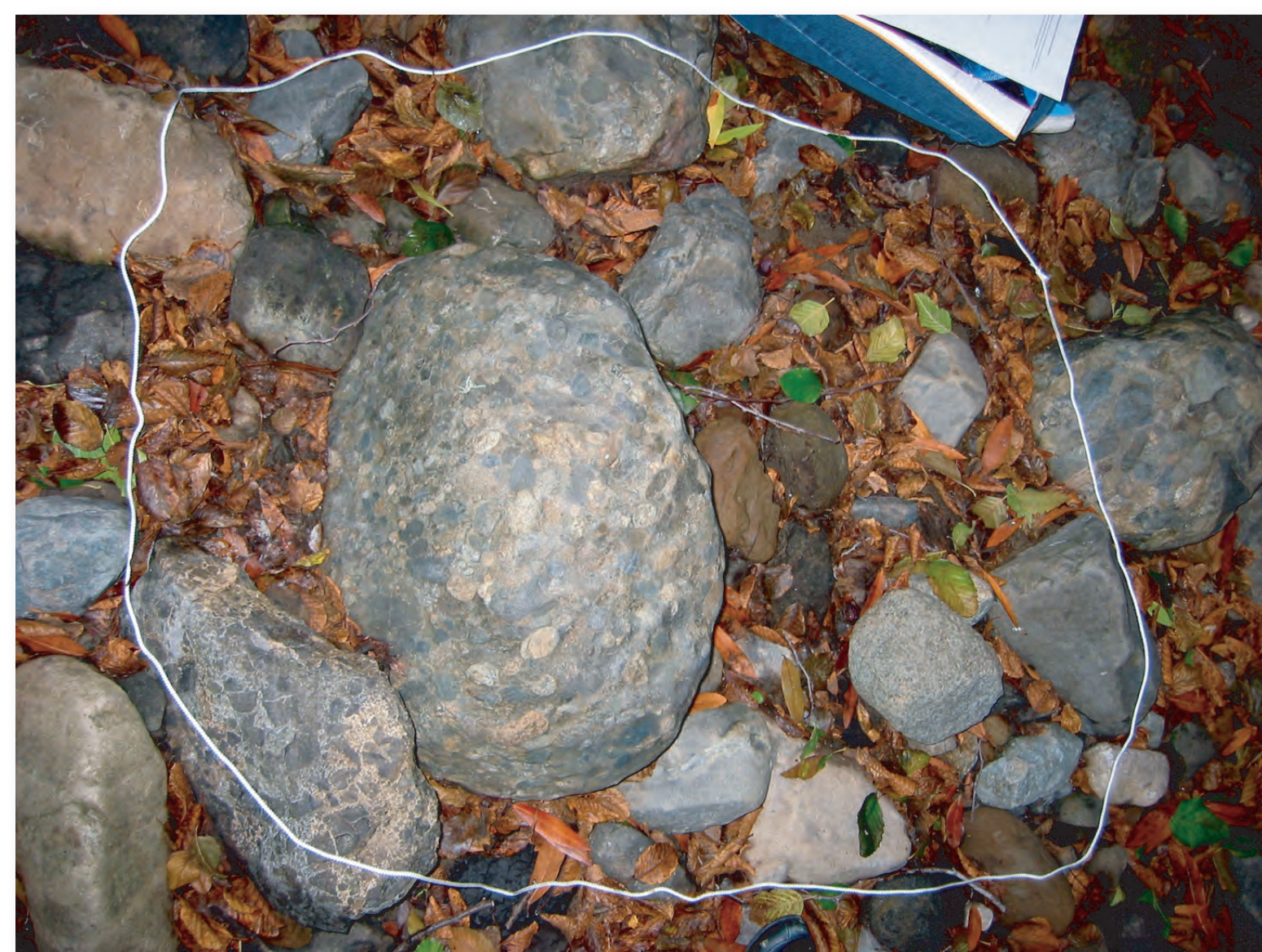
Measuring the five largest clasts in a 1 m square area
