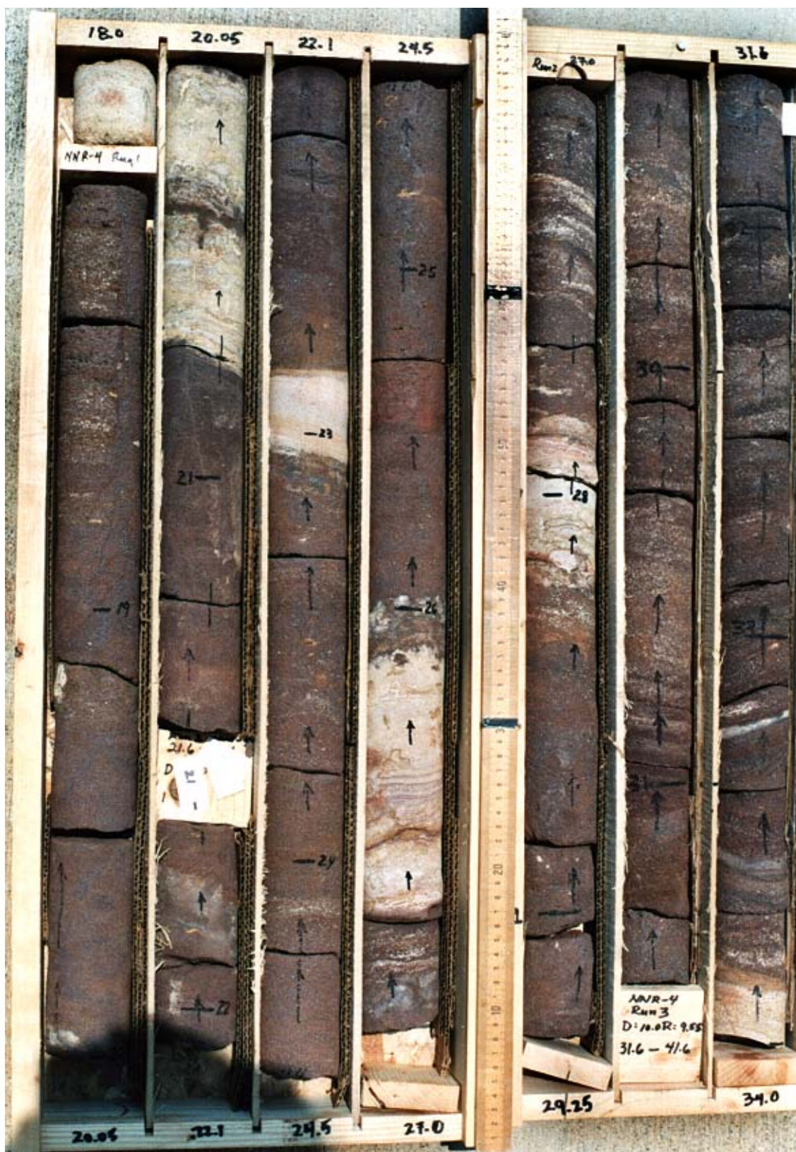
Figure 6: Core photograph of the Upper Hickory (0-50' below surface).
