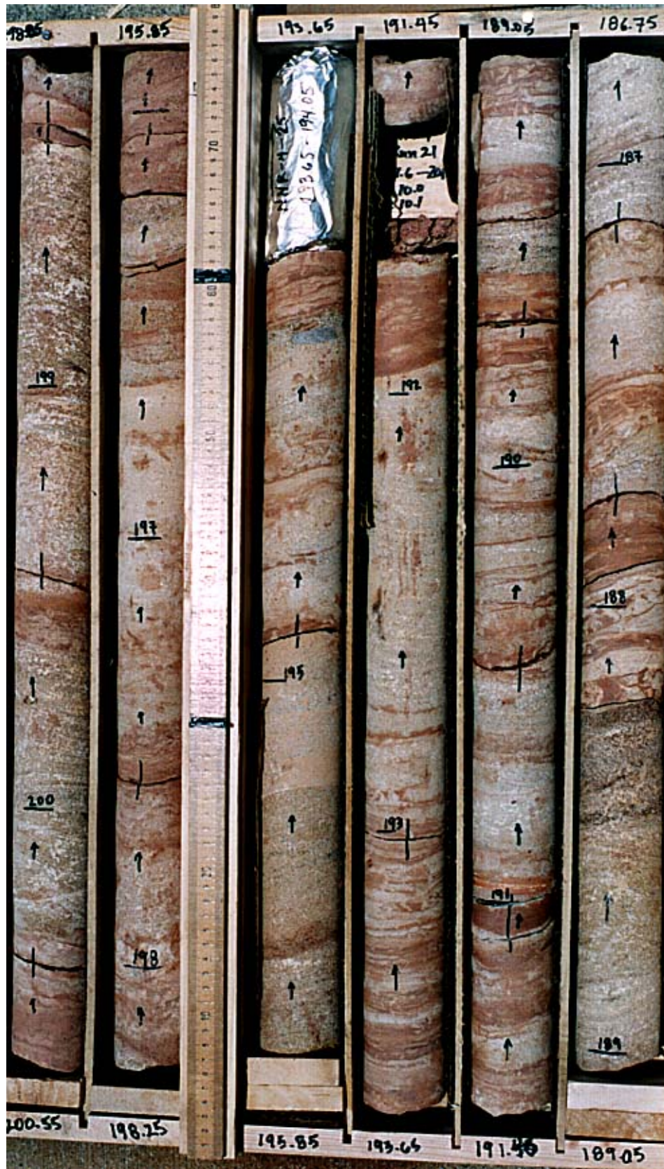
Figure 4: Core photograph of the Lower-Middle Hickory (135-250' below surface).
